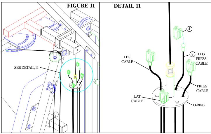
Run the LEG PRESS CABLE through the correct hole on the d-ring and attach one KEYHOLE CLEVIS to the end of the LEG PRESS CABLE. See FIGURE 11 & DETAIL 11. (NOTE: If the 445101 SECOND STACK kit is installed, evenly space the LAT & LEG EXT. CABLES on the D-RING)
